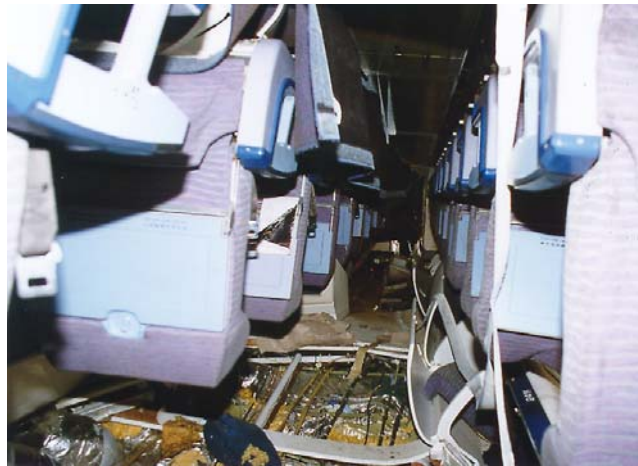
Above : Absence of gangway inside the overturned fuselage
